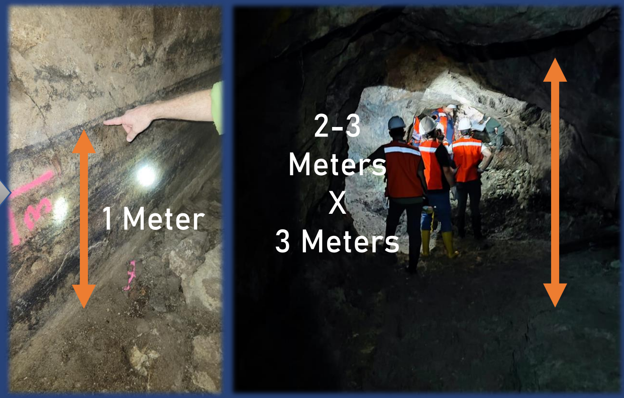
From Promontorio entrance at haulage level to 600m towards Balvanera shaft has been successfully dewatered Access to workings within 2 x 3 meter adit
