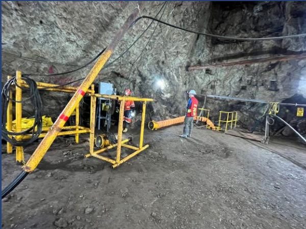
Balvanera shaft hoist room. Note yellow safety railing around Balvanera shaft collar at center-right of image and gray electrical control panel in center-left background. Orange air duct leads into shaft to provide ventilation. Steel casing slanting from right to left in left foreground contains electrical cable from for lighting and welding and other tools. The wooden beam above the shaft collar is a vestige of historical hoisting equipment.
