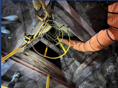
Balvanera shaft hoist room. Note yellow safety railing around Balvanera shaft collar at center-right of image and gray electrical control panel in center-left background. Orange air duct leads into shaft to provide ventilation. Steel casing slanting from right to left in left foreground contains electrical cable from for lighting and welding and other tools. The wooden beam above the shaft collar is a vestige of historical hoisting equipment.
