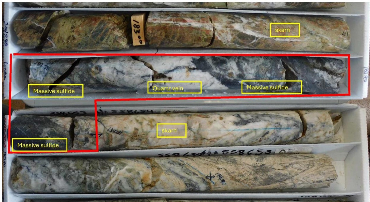
Figure 1. Drill core photo of Hole AL24-105: 182.80 m – 185.10 m, intersected 1.25 m of 309 g/t AgEq including 0.70-m interval (183.35 – 184.05 m) that assayed 2,976 g/t Ag Equivalent or 2,431 g/t Ag, 0.266 g/t Au, 1.29% Cu, 7.41% Pb, and 6.06% Zn . Host rock is skarn-altered limestone.
